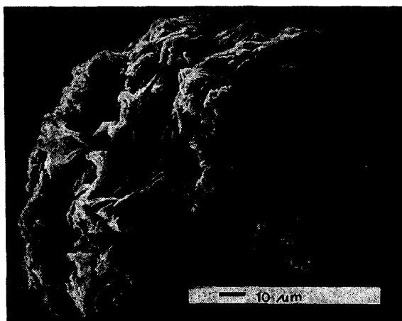
5-1 The Scanning Electron Micrograph of Decomposed Organic Matter of Sapric Peat after Boiling with 1 M NaHCO 3
